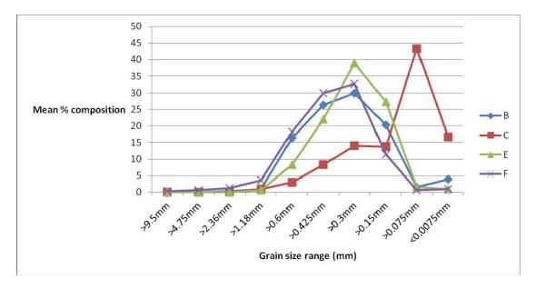
Figure 4 - Particle size distribution chart for sites B, C, E and F
