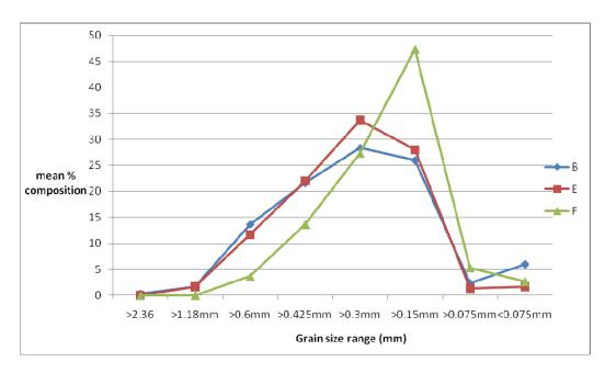
Figure 5 – Comparative Particle size distribution chart for sites B, E and F from Autumn sampling
