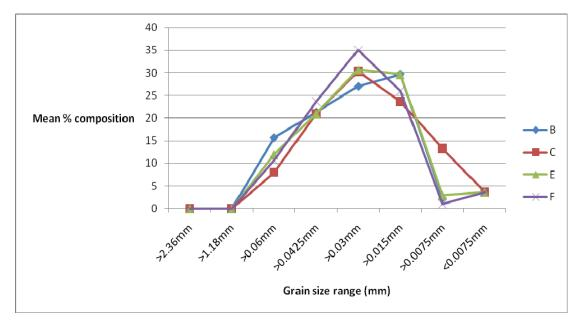
Figure 4 - Particle size distribution chart for sites B, E and F
