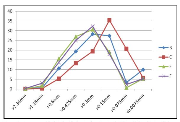
**Figure 5 –** Comparative Particle size distribution chart for sites B, C, E and F from Spring 2014 sampling
