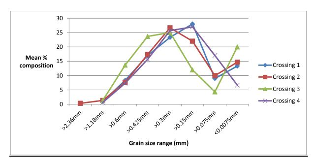
Figure 3 – Mean grain size distribution for creek crossings (comparison from baseline monitoring undertaken in April 2014)
